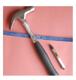
Punch two holes at the marked points. Make the first hole as big as the screw posts diameter for the button stud. Make the second hole slightly bigger than the shaft of the button stud.
