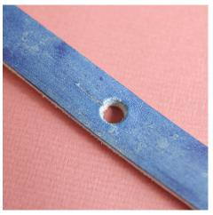
With an X-acto knife, cut a 1/4 inch slit. This is to allow the stud to go through the small hole. You may have to open up the slit to allow the stud to go through easily.
